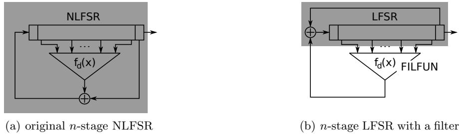
Fig. 3: Schematic of an NLFSR represented as an LFSR with a filter FILFUN
